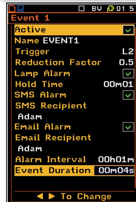
**Trigger** is set to DIN 4150-2, the building type, marked as Line 2 (L2).
