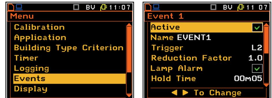
Event can trigger Alarm Lamp, Email or SMS. It is important to set up the event duration for the length of observed vibration activity - for example 5 to 10s for train passage. To browse events on the screen use UP/DOWN arrow in BS 7385-2 view.
