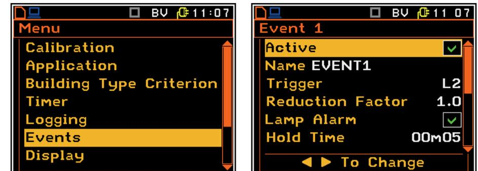
Event can trigger Alarm Lamp, Email or SMS. It is important to set up the event duration for the length of observed vibration activity - for example 10s for train passage. To browse events on the screen use UP/DOWN arrow in DIN 4150-3 view.
